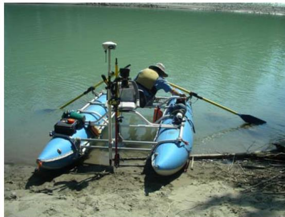
Fig. 2 Hydrographic survey equipment.
